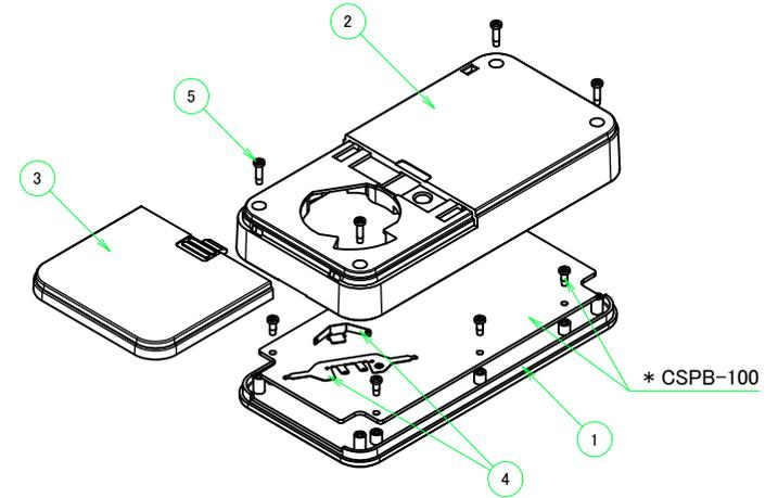
**電池構造 / Battery compartment type**
