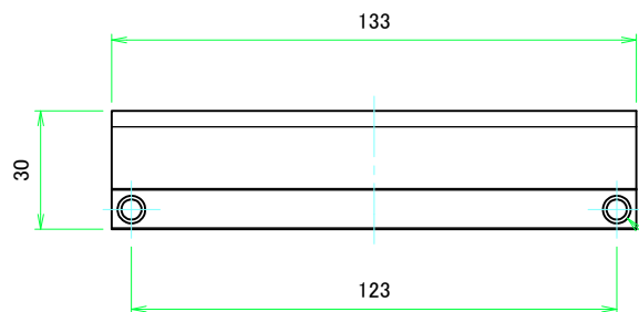
2-M4用サラ穴 2-M4 Countersunk
